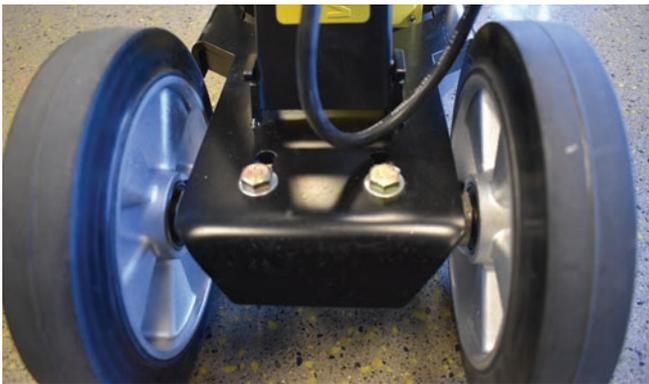
Once head has been converted, loosen the bolts on the rear of the machine. Move the wheels in the desired position and retighten the bolts ensuring they are secure enough to run the machine.
