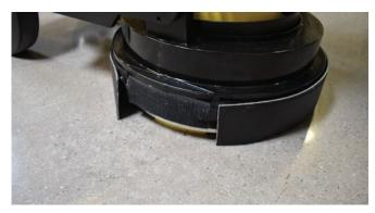
Once head has been converted, loosen the bolts on the rear of the machine. Move the wheels in the desired position and retighten the bolts ensuring they are secure enough to run the machine.
